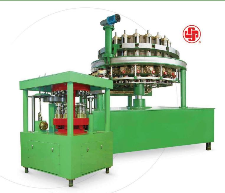
> Automatic Filling/Seaming Machine For Large Cans
